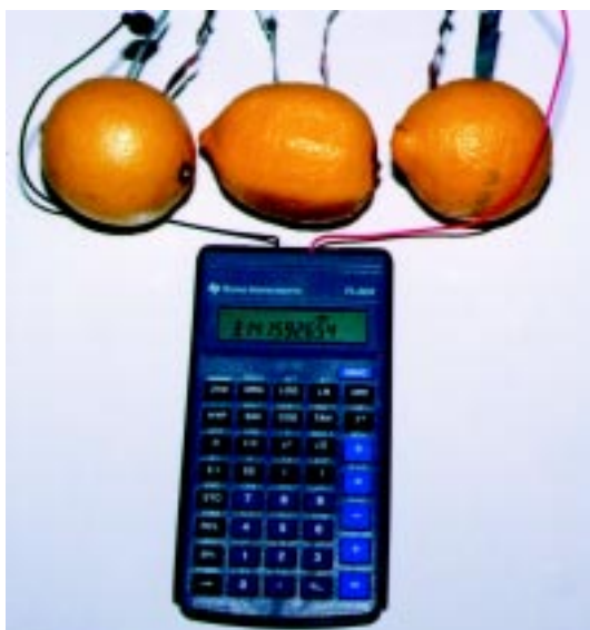
Figure 1. Lemon pi! The TI-30 calculator powered by three lemon cells.
